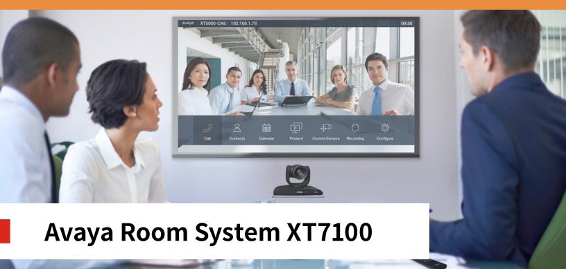
The Avaya Room System XT7100 is the flagship offering in the XT series of video conferencing room systems. The XT7100 incorporates H.265 High Efficiency Video Coding (HEVC), one of the industries most advanced video compression technologies. H.265 HEVC doubles the video compression efficiency of H.264 High Profile, enabling full HD 1080p 60fps video with half the bandwidth required<sup>1</sup>, delivering an exceptional experience with a total lower cost of ownership.
