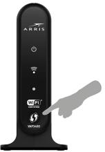
4. The Client's Wireless Link LED lights: Nou have now established a secure wireless connection between the Access Point and the Client. Check to ensure the Wireless Link LED lights, indicating the VAP is functioning as a Client. You now can begin streaming video content to your set-top box or boxes.
