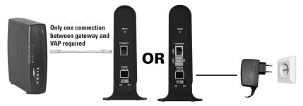
3. Connect the power adapter to the VAP, plug the adapter into a wall outlet and set the Power switch to the ON position. You'll see the Power LED on the unit's front panel light green, indicating the unit is powered.
