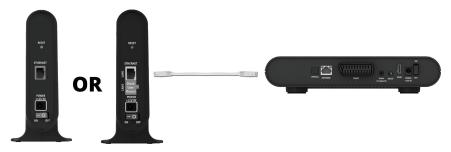
Connect the power adapter to the VAP, plug the adapter into a wall outlet and set the Power switch to the ON position. You'll see the power LED on the unit's front panel light green, indicating the unit is powered.
