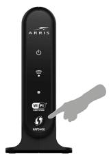
4. After the VAP establishes a wireless connection with your set-top box, the Wireless Link LED lights: \_\_\_\_\_. Check to ensure the Wireless Link LED lights, indicating the VAP is functioning as a Client. Your VAP is now ready to stream content to the device equipped with the VAP adapter.
